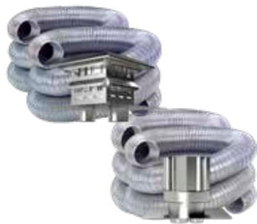
Co-Linear Vent System Z-FLEX® DVI Kits designed for use when converting existing wood-burning fireplaces into gas. Allows for a completely sealed system that does not compromise indoor air quality. Kit includes two Triplelock® Gas Liners, one for flue exhaust, the other for outside combustion air. Includes either extreme weather or decorative co-linear termination options
