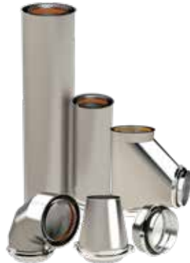
Z-VENT® Single or Double Wall AL29-4C Stainless Steel rigid vent for Category II, III, & IV vent in 3" to 24" diameters with revolutionary double fail safe seal that dramatically reduces the installed vent time and cost.
