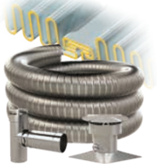
Z-VENT® Smoothcore™ AL29-4C Stainless Steel flexible vent with smooth inside diameter for Category II, III & IV vent, in 2" to 8" with patented airtight Triple-Lock Construction & exclusive ZLOK Tee.
