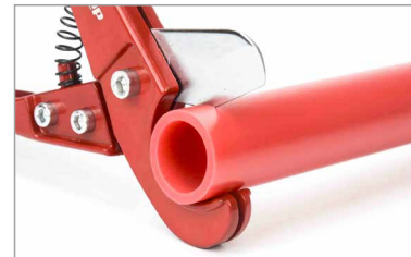
1.Cut the pex pipe square, leaving a clean, even edge. Remove burrs.
