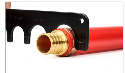
4.Measure the crimped ring with Go-No-Go gauge(included).
