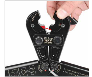
3.Lift up the fixing pin and take out the inserted jaws.
