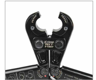
6.Replacement is finished. Make sure that the jaws are installed correctly, improper installation will break the screw.
