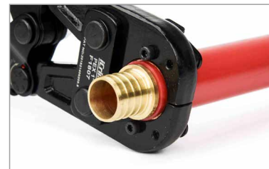
3.Choose correct jaw size. Position the pipe with copper ring part into the jaw and crimp.
