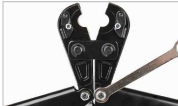
2.Looseen LH or RH "back nut" with wrench, turn only any one "adjustment dials" one increment or reduction at a time.
