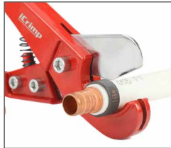
Step 1: Cut the pipe as close as you can to the fittings
