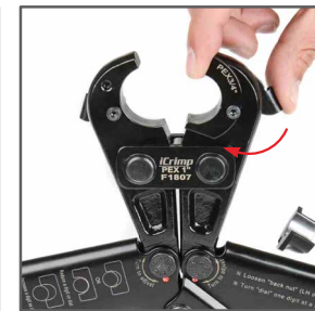
5.Lift up the fixing pin and push into the inserted jaws with correct size you needed. Push back the hook.
