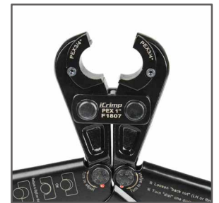
6.Replacement is finished. Make sure that the jaws are installed correctly, improper installation will break the screw.
