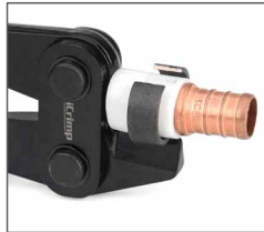
Step 3: Rotate 180° and cut again (2-4 times cut required)
