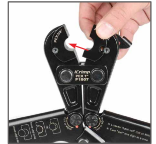
3.Lift up the fixing pin and take out the inserted jaws.
