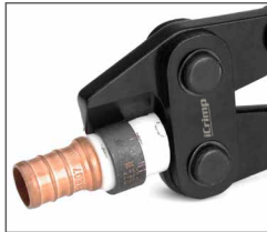
Step 2: Position the removal tool and cut
