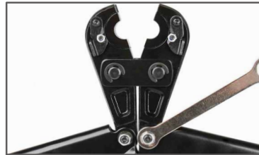
2.Loosen LH or RH "back nut" with wrench, turn only any one "adjustment dials" one increment or reduction at a time.
