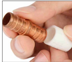
Step 4: Remove copper ring and take out the fitting from the pipe
