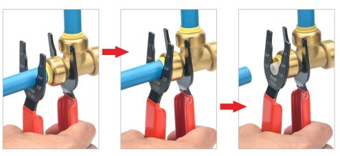
Step 1: Place the teeth around the fitting assembly. The fork end with the iCrimp logo should be positioned around the tube to against the release collar and the other end around the neck of the fitting.
