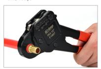
3. Align the jaws with copper ring and compress handles to fully close the jaws.
