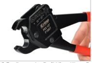
2. Pull up the upper handle slightly and then pull upper handle backward, hold both handles with one hand to keep the jaws open.
