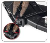
1. Remove "C" clamp with screwdriver.
