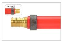
1. Cut tubing end squarely. Slide crimp ring over end of tubing. Insert fitting into end of tubing until it stops.
