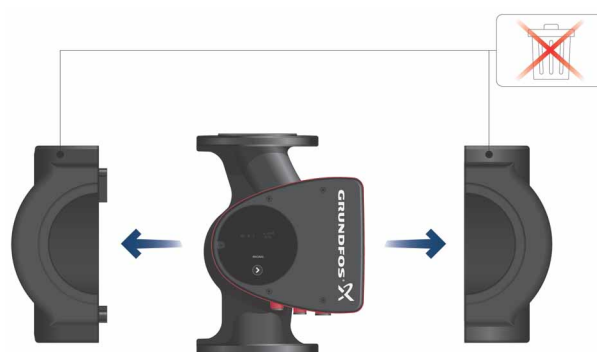
Fig. 3 Fitting insulating shells to the pump
