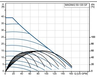
Pumped liquid = Water Liquid temperature during operation = 140 °F Density = 61.35 lb/ft³
