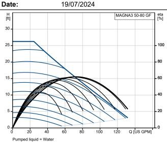
Liquid temperature during operation = 140 °F Density = 61.35 lb/ft³
