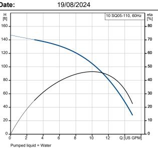
Liquid temperature during operation = 68 °F Density = 62.29 lb/ft³
