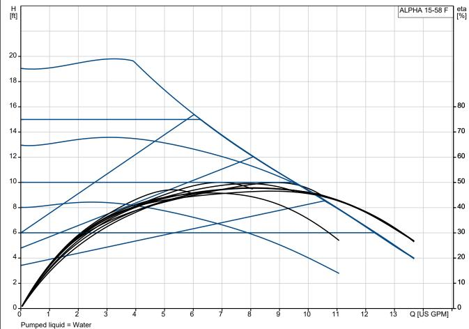
Pumped liquid = Water Liquid temperature during operation = 140 °F Density = 61.35 lb/ft³
