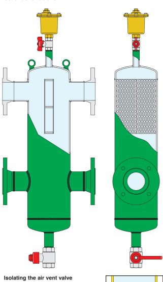
In flanged separators, the air vent is isolated manually, using a shut-off ball valve. In union separators, however, the air vent body is automatically isolated by the check valve, which closes when the air vent body is removed.
