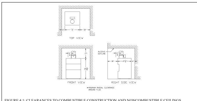
FIGURE 4.1: CLEARANCES TO COMBUSTIBLE CONSTRUCTION AND NONCOMBUSTIBLE CEILINGS, WALLS, AND DOORS.
